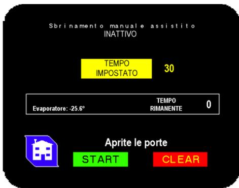
After you have set the machine on OFF and taken off all the product from the cell, open one door and run the program by pressing START. The temperature of the evaporator and the time will be shown. Anyway, if you decide to stop the operation just touch the button clear. Meanwhile the operation is running you can take a look to other menus.
