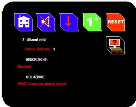
The **Alarms** menu is the main page to enter and manage alarms. On the top left active alarms will be shown, then looking down on the screen you will see the alarm's index with its description and solution. If there are multiple alarms, you can cycle through the various
