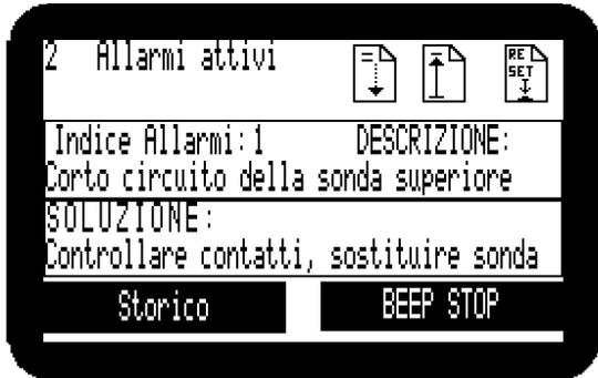
The **Alarms** menu is the main page to view and manage alarms. In the upper left it displays the number of active alarms, then below are displayed respectively the active alarm with description and its solution. If there are multiple alarms, you can see all alarms
