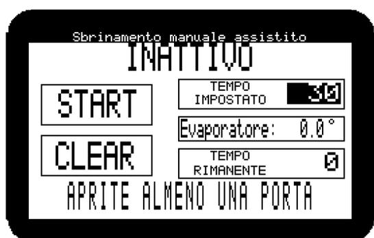
After placing the machine on OFF mode and emptied the cell from products, open at least one door. Start the program by pressing the START button. This will display the temperature of the evaporator and the remaining time to the end. In any case, if you decide to stop the operation will be sufficient to press the CLEAR button. During the operation, you can view other menus.
