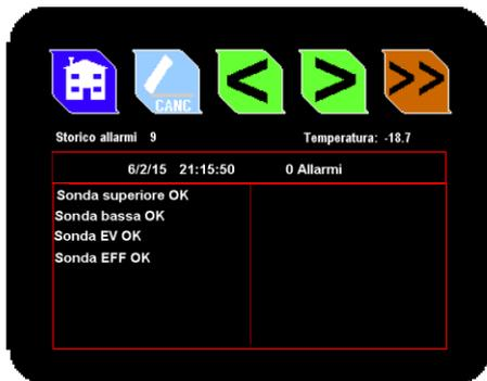
The PLC director over the alarm log all the events of return from alarm, therefore the latest history should be the last state of the machine when the alarm. By the buttons <> you can enter former and later events, but by >> you will see the latest.
