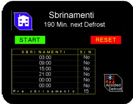
By entering this page you can activate and set up programmed defrost. The activation of just one programmed defrost, will exclude automatic defrost. You can set up to 6 programmed defrost, by choosing hour, minutes and/or seconds and pressing **Yes** next to where the time is shown.
