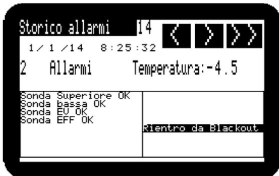
The PLC, as far as the alarm history, detects all the events of fall and return alarms, therefore the last screen should be state the last alarm of the machine. Use <> so you can view the events before and after and with the >> button you will reach directly the last alarm occurred.
